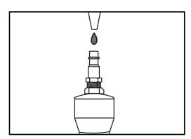
Figure 6. Lubricating nailer via air inlet.
